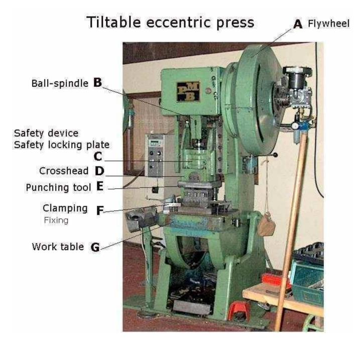
Ball-spindle Ball-spindle = kuglespindel
